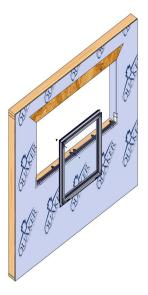
Install the first window unit in place following the QWP standard nail fin installation guide. Make sure the unit doesn't have a nail fin on the side of the unit where the mull will go.
