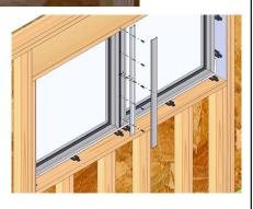
Apply sealant up the bottom 6" of the center of the T-mull filling the entire area as shown above.
